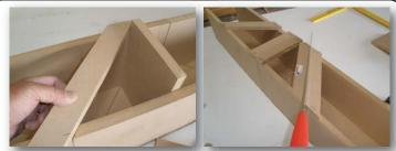
Using a piece the same width as your base, space the sides of the box apart. Line up cross braces with your angle cuts and secure to the box.
