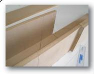
Start dry fitting all of your angle cut pieces, making sure they stay lined up with your base marks. They should be spaced the width of the new saw blade.
